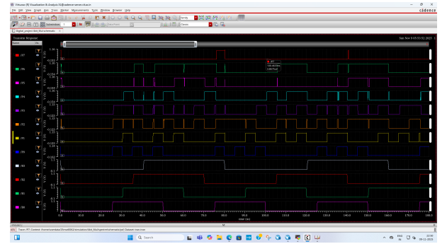
Fig. 9: 4-bit array multiplier result waveform
